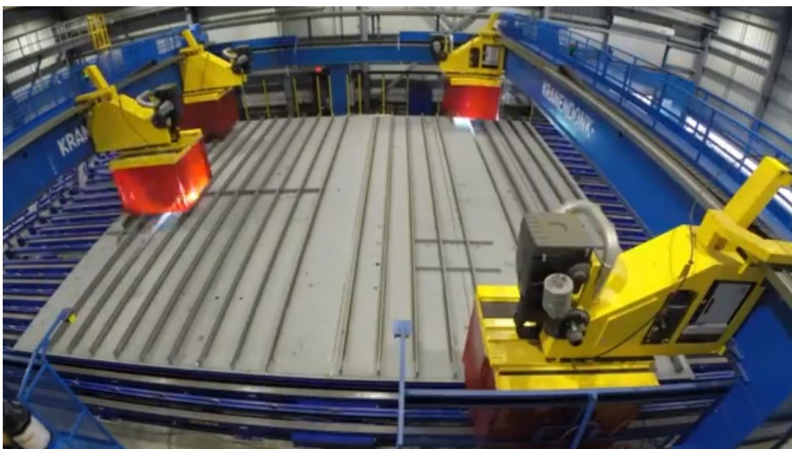
Figure 3-2. NASSCO Thin Panel Plate Line Operation
